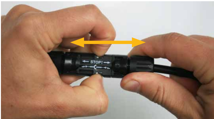
Fig. 5: Disconnecting an MC4 type connector by hand (Multi-Contact or Hosiden)
